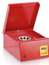
Gambar 2 *Butyrometer* Gerber *centrifuge*
